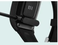
The charging cable attaches to the back of the watch and clicks into place via magnets.
